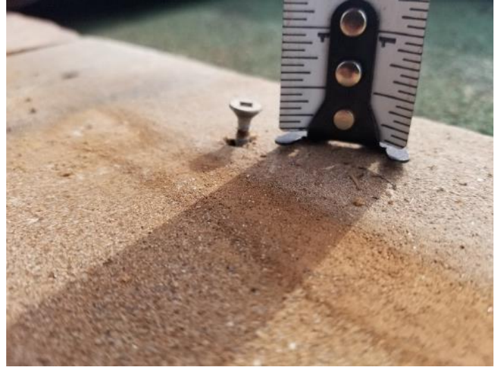
Photo 14: Fastener withdrawn & damage to fastener hole at Bldg 30
